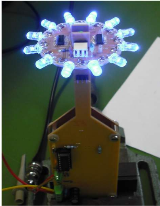
Figure 3.20: Used planar emitter
